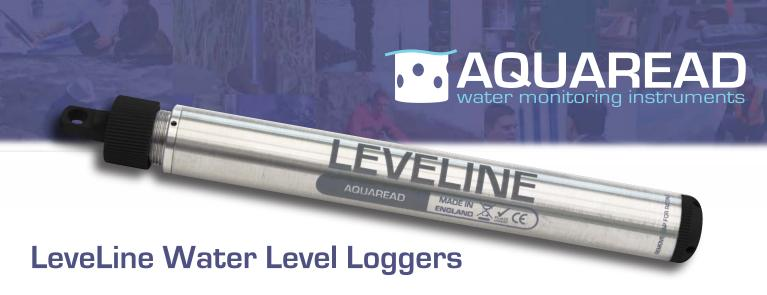
The LeveLine records highly accurate water level and temperature measurements in groundwater and surface water applications. Housed inside an all titanium body is a ceramic level sensor, temperature sensor, 10-year lithium battery and a versatile datalogger with capacity for 500,000 data points.
